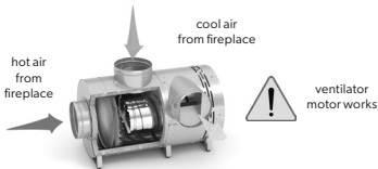
Fig 1.b. Temperature in fireplace hood is high (between 70 and 180 °C)
